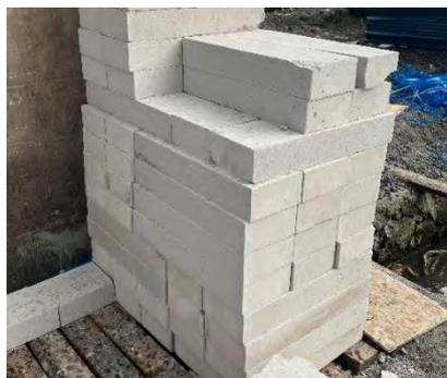
Gambar 1. Material Bata Ringan AAC
