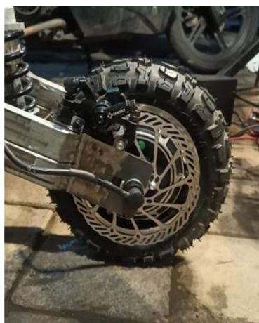
Figure 1. Electric scooter with a 36V 40-watt BLDC
