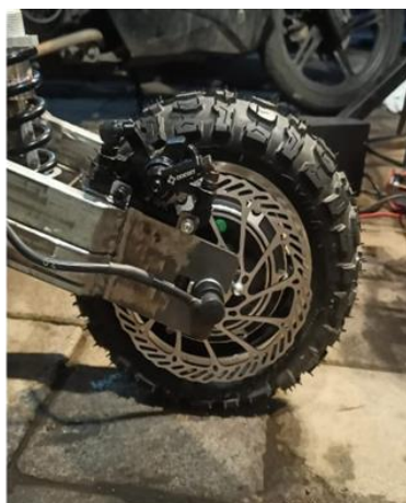
Figure 1. Electric scooter with a 36V 40-watt BLDC
