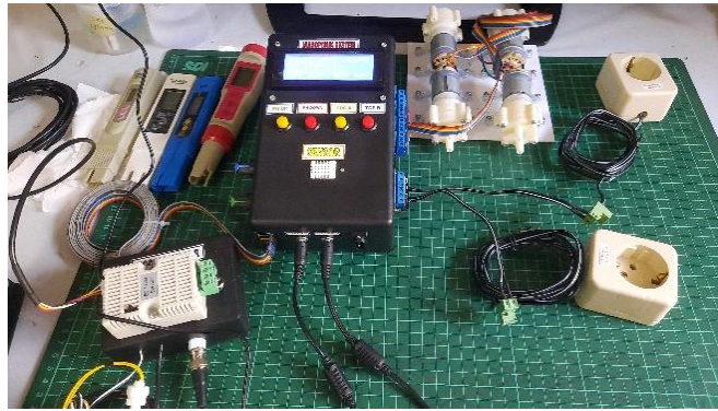
Figure 4. Hardware Monitoring of Smart Farming-based IoT
