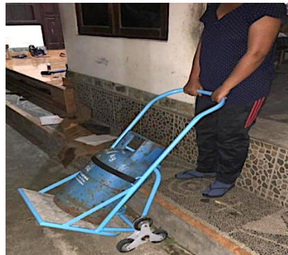
Figure 3. Lift and transport 12 kg LPG with conveyance
