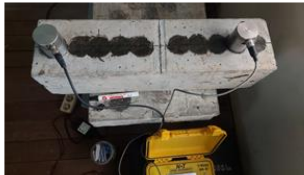
Figure 4. Instrument set up for T-Method
