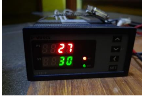
Figure 3. Set the Thermo control at room temperature
