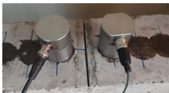
Figure 2. Instrument set up for BS method
