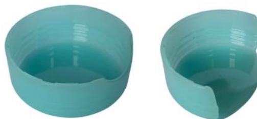
Figure 1. Short shot defect in injection molding cover pot
