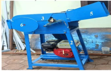
Figure 4. Flywheel model organic waste shredder
