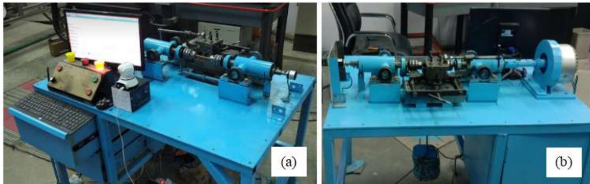
Figure 4. Construction of the integrated rotating bending fatigue test machine: (a) Front view, and (b) Rear view
