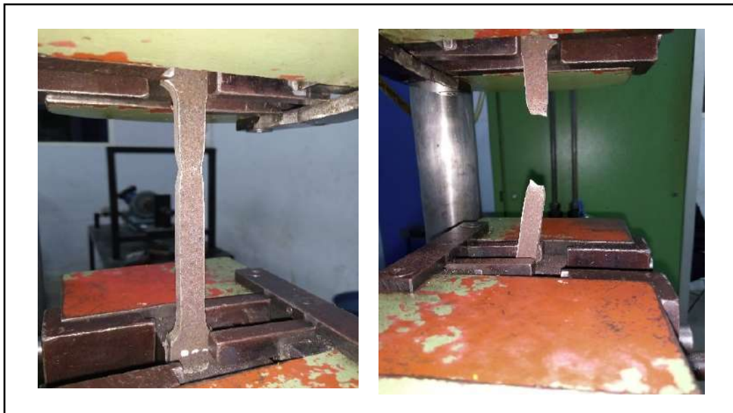
Figure 6. Tensile strength testing process
