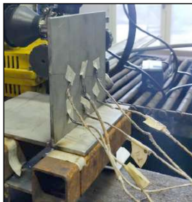
Figure 2. Tackwelded Specimens and Installed Thermocouples
