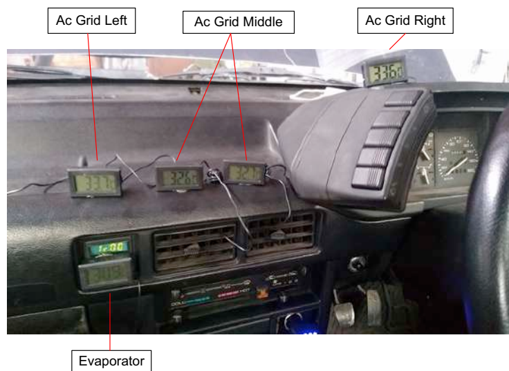
Figure 3. Cooling rate data collection process
