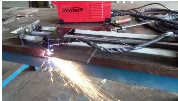
Figure 7. Testing of 1 axis plasma cutting mechanism
