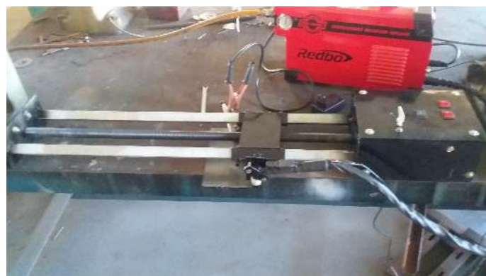
Figure 6. Re-checking the electrical installation before trying it
