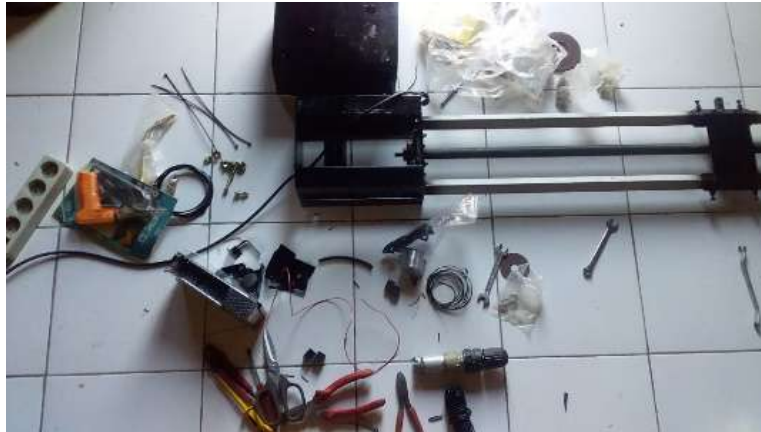
Figure 4. Assembly of components, bracket rails, frame, drive screw shaft, bracket
