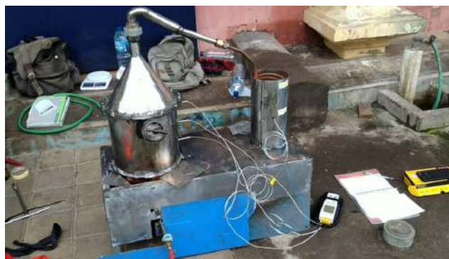
Figure 1. Setup pyrolysis of LDPE plastic
