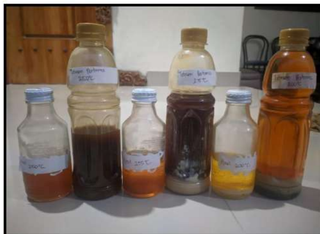
Figure 3. Pyro-oil product with different pyrolysis temperature
