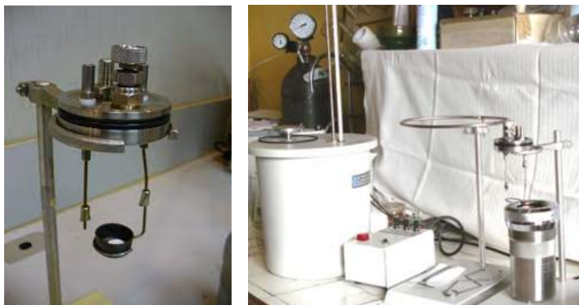
Figure 2. Standardization of bomb calorimeter using benzoic acid.
