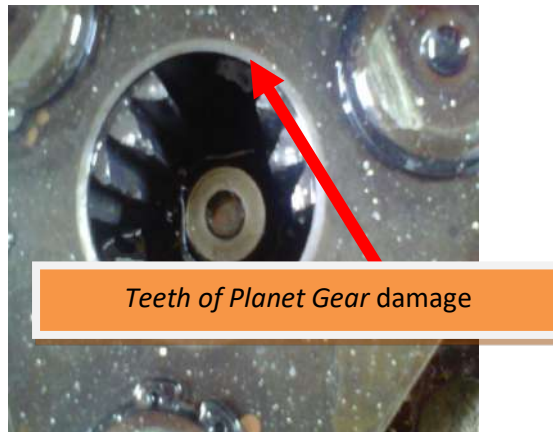
Figure 11. Planet Gear Broken
