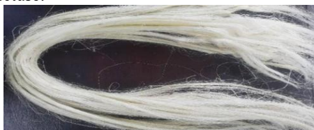
Figure 3. Raw banana fiber used as natural adsorbent before filtration process
