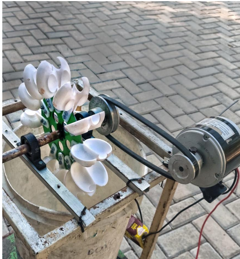
Figure 3. Turbine & Generator DC
