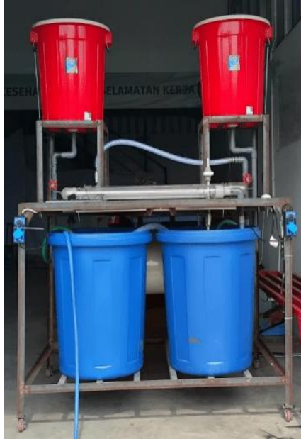
Figure 4. Fabrication of heat exchanger
