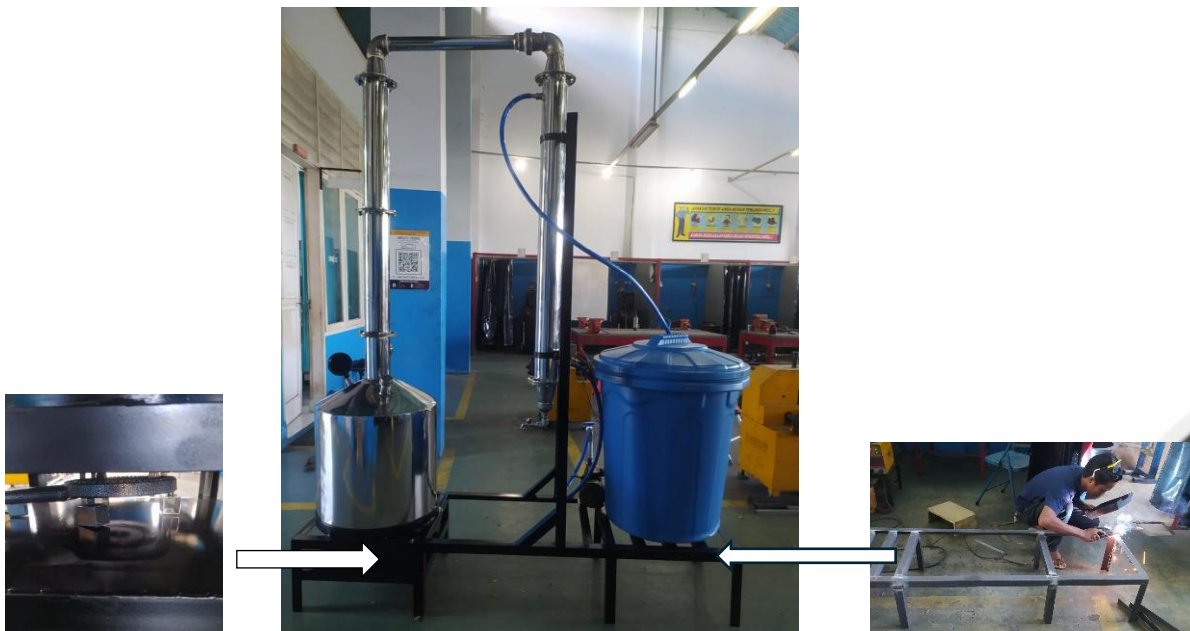
Figure 4. Design results of bioethanol distillation-dehydration equipment
