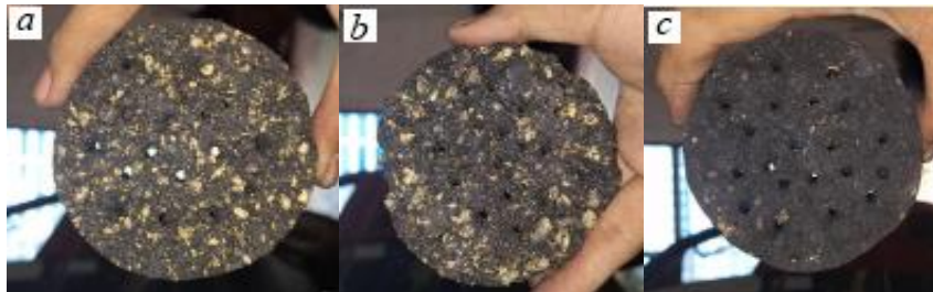
Figure 1. Catalytic converter from dry corn cobs and corn cob charcoal: a. Charcoal 50%, b. Charcoal 70%, c. Charcoal 100%
