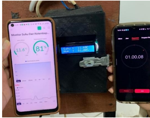
Figure 5. Data transmission to the Blynk application
