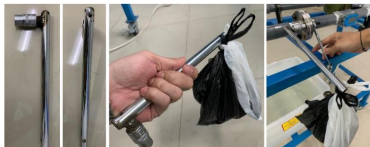
Figure 5. Creation of torque measurements smaller than 5 Nm which are not available in the trade
