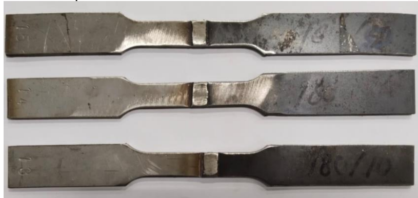
Figure 1. ASTM E8M standard test specimen
