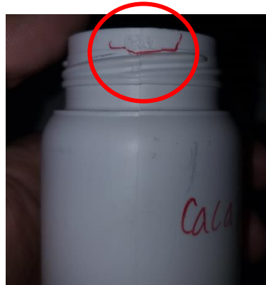
Figure 17. Rough joint line defect
