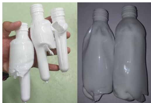
Figure 16. Failure to blow
