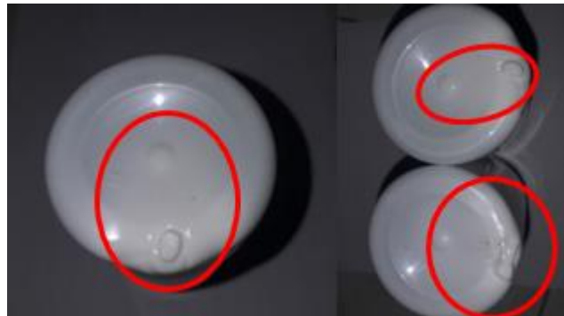
Figure 15. Slanted navel point (Off center base)
