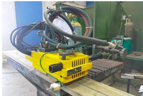
Figure 4. Gas Cutting Machine for Constant Travel Speed
