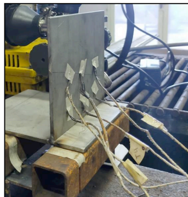
Figure 2. Tackwelded Specimens and Installed Thermocouples
