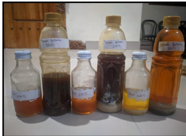
Figure 3. Pyro-oil product with different pyrolysis temperature
