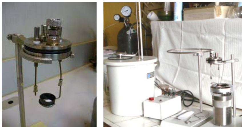
Figure 2. Standardization of bomb calorimeter using benzoic acid.
