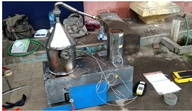
Figure 1. Setup pyrolysis of LDPE plastic
