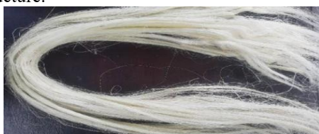
Figure 3. Raw banana fiber used as natural adsorbent before filtration process
