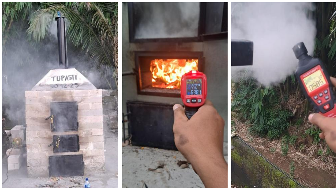
Figure 2. Existing image of a simple incinerator made from lightweight bricks and the combustion process as well as measuring temperature and CO levels.
