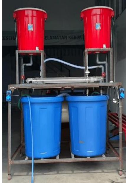
Figure 4. Fabrication of heat exchanger
