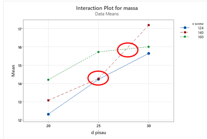
Figure 9. Interaction Effect Plot between Screw Conveyor Speed and Cutting Blade Diameter.
