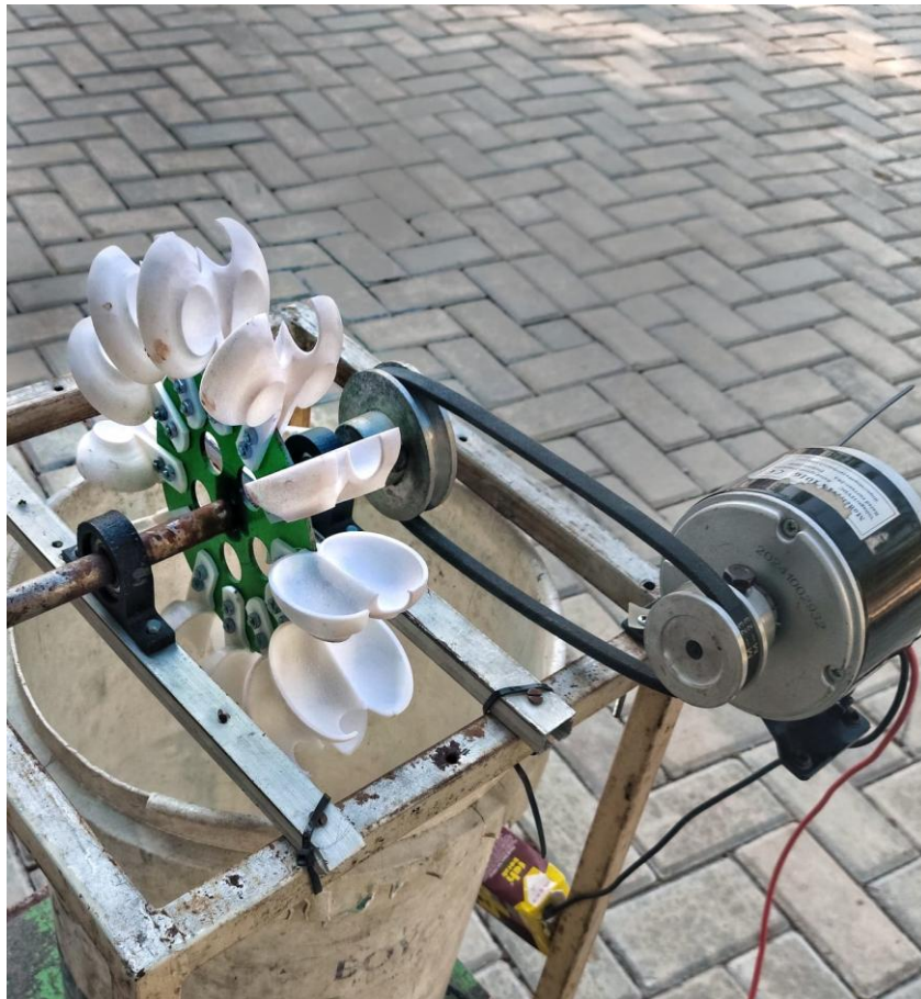
Figure 3. Turbine & Generator DC
