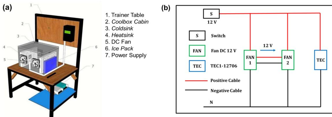
Figure 1. (a) Construction of the thermoelectric coolbox system and (b) electrical wiring diagram for the thermoelectric system
