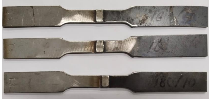
Figure 1. ASTM E8M standard test specimen
