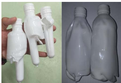
Figure 16. Failure to blow
