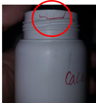
Figure 17. Rough joint line defect
