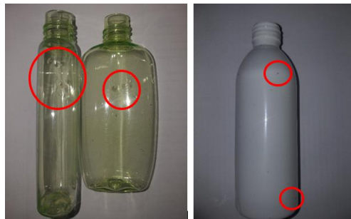
Figure 8. Black Spot Defect
