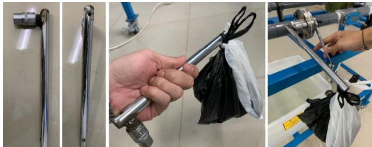
Figure 5. Creation of torque measurements smaller than 5 Nm which are not available in the trade
