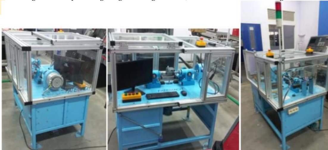
Figure 2. Fatigue Testing Machine, FATEMACH, Left Side View, Front View, and Right Side View
