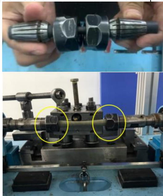
Figure 3. The shape of the collet nut and its installation on the spindle
