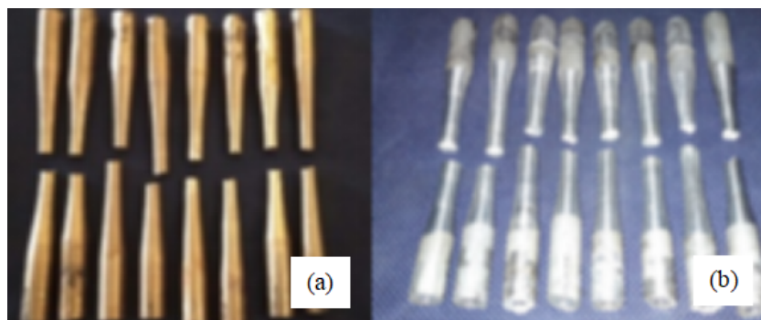
Figure 6. Specimens after fatigue testing: (a) Brass, and (b) Aluminium
