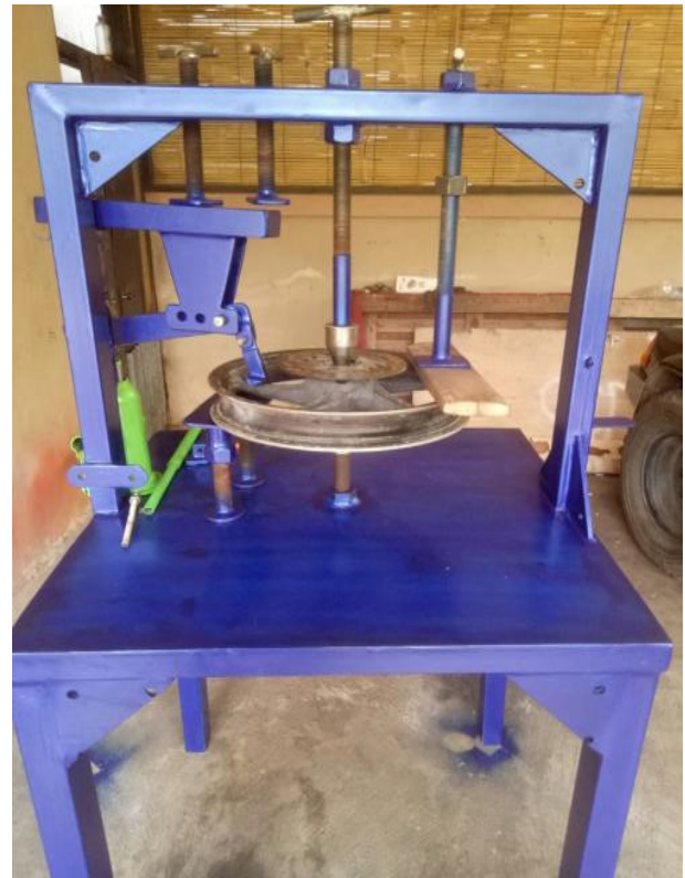
Figure 8. Motorcycle wheel rim press tool
