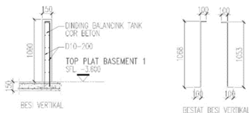
Gambar 3. Detail Penulangan Dinding Balancing Tank
